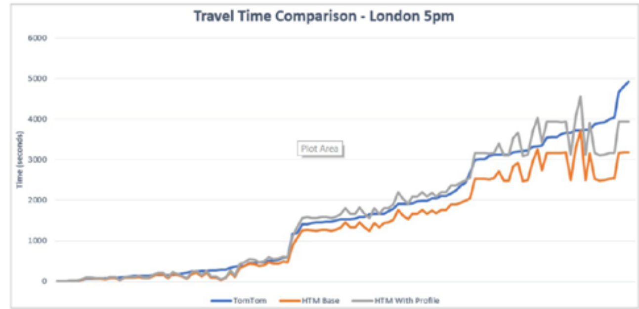
Travel times at rush hour in London, comparing results from HTMs with and without travel area weightings profile. TomTom data used as a baseline.
